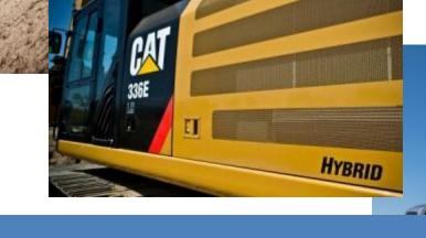
Caterpillar employs hydraulic hybrid technology that is 98% common with the conventional 336E excavator to boost fuel efficiency of the 336EH hybrid 50%.
